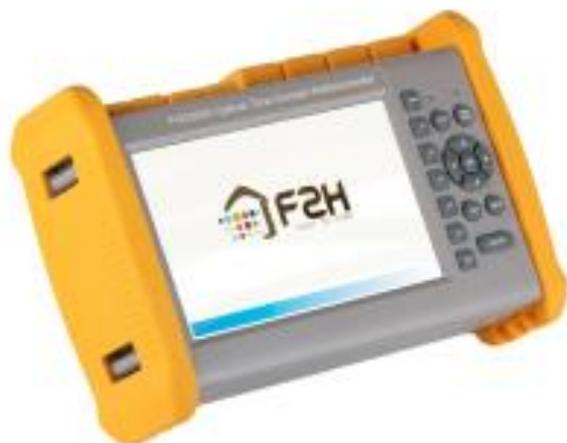
FHO5000 Series Optical Time Domain Reflectometer (OTDR) is an intelligent meter of new generation for the detection of fibre communications systems.
