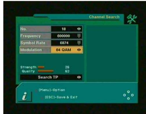
Use ◀▶ keys to select “Search TP” after parameters are set. PDSR-3000P-XXC could search for TV and radio channels automatically. During searching procedure, you can see a list of the previously searched channels in the Searched List Box on the screen. On completion of searching channels, the cursor will be moved to “VIEW” automatically, then press OK key to watch the program.
