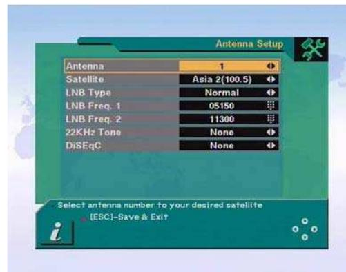
5. Switches ( 22KHz, DiSEqC ) : you could select the switches with which you want to configure the antenna.
